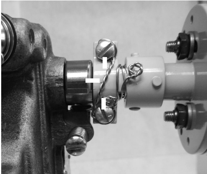
Figure 5-11f: Application of Anti-Sabotage Lacquer
